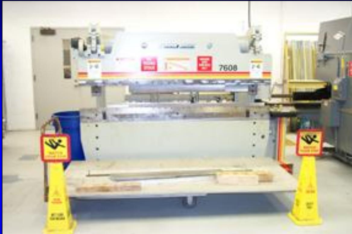
A brake is used to bend sheet metal.
